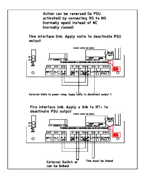
Terminal SQ is a 100ma output that bypasses the output fuse, which can be used to indicate a fault condition with a buzzer\* or LED via the fault relay contacts.
