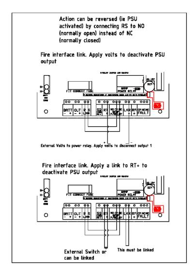
Terminal SQ is a 100ma output that bypasses the output fuse, which can be used to indicate a fault condition with a buzzer\* or LED via the fault relay contacts.
