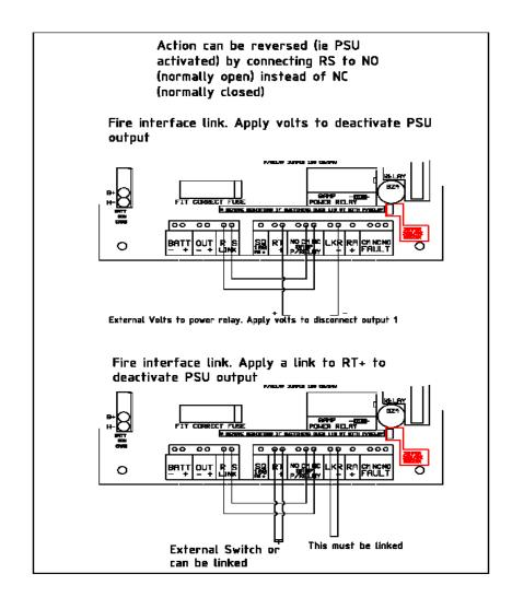
Terminal SQ is a 100ma output that bypasses the output fuse, which can be used to indicate a fault condition with a buzzer\* or LED via the fault relay contacts.
