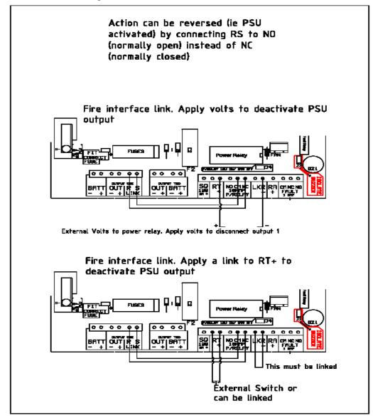
Terminal SQ is a 100ma output that bypasses the output fuse, which can be used to indicate a fault condition with a buzzer\* or LED via the fault relay contacts.
